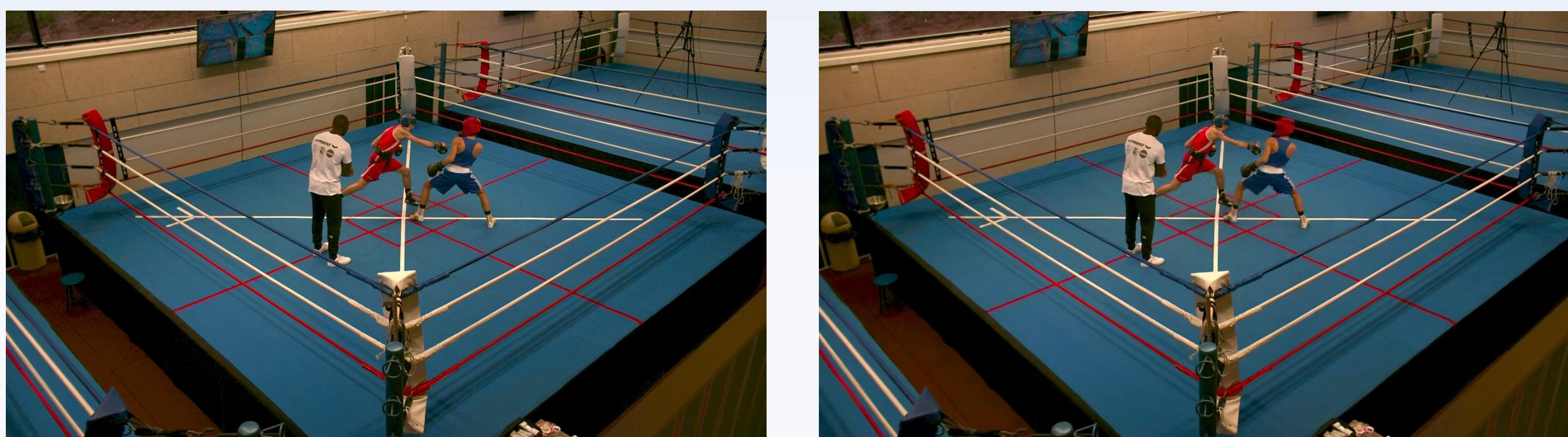
Fig. 1. Comparison between 2 frames of a given moment of the match - Left: Reference video - Right: Compressed video encoded at 500kb/s.
