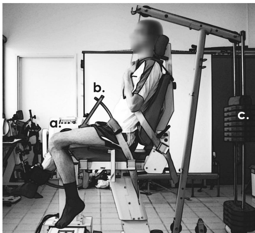
Fig. 1. Picture of the device. A plate-loaded resistance training device was integrated to an isokinetic dynamometer Biodex System 3 (a). Loads (c) were linked to the dynamometer attachment by a wire. The wire passed through two pulleys and followed a half-circle metal piece (b) fixed to the dynamometer attachment. (a) Dynamometer – Biodex System 3 Pro; (b) half-circle metal piece; (c) loads.
