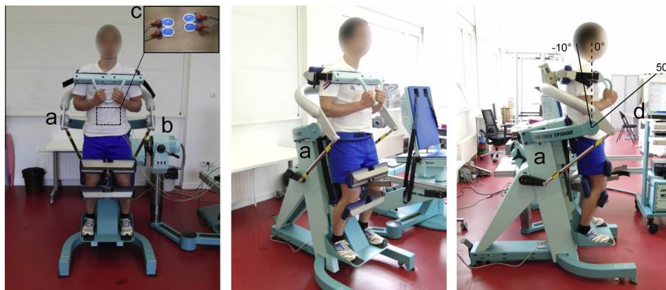
Fig. 1. Experimental set-up. Frontal (left picture), three-quarter (middle picture) and lateral (right picture) view of the Con-Trex TP-1000 module (a) connected to the isokinetic motor (b). Surface electromyographic activity of rectus abdominis (c) and erector spinae was synchronously recorded with mechanical data provided by the dynamometer, which was driven by a dedicated computer (d). Trunk extensions and flexions were executed from -10^\circ to 50^\circ ( 0^\circ = vertical position).
