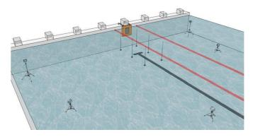
Fig. 1. 3D kinematic calibration system and camera set-up. The two cameras that were close to the turning wall were about 0.7-m deep. The two following cameras (from the turning wall to the other end of the pool) were placed as deep as possible (pool depth). The fifth camera was placed in a center lane of the pool and was about 1.5-m deep. The angle between each pair of consecutive cameras ranged from 451 to 601.
