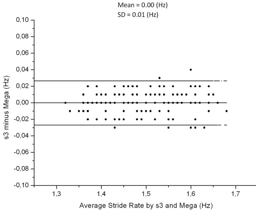
**Fig. 2** Bland–Altman plot depicting the calculated bias between the two devices of measurement and the limits of agreement for stride rate measurement using the s3 accelerometer (n=153).
