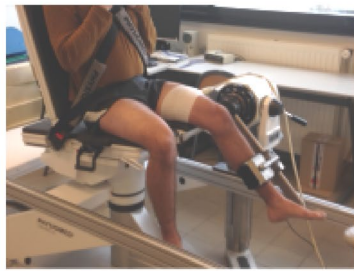
Isokinetic conditions 2 × 4 velocities 100, 200, 300 and 450°.s -1
